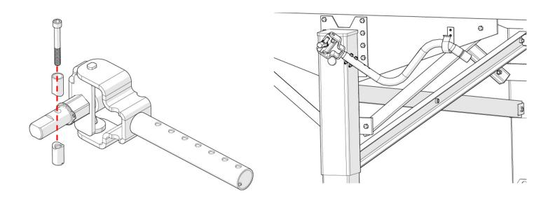
**B. INSTALL ACTUATOR ON CROSS SHAFT**
